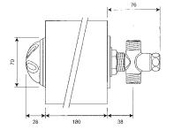
TBV/ADJ/180 **Application**For up to 180mm wall thickness.
