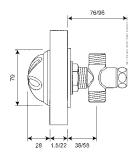
Order Code TBV/ADJ/22 Application For 1.5mm – 22mm wall thickness. Fixing 3/4" BSP. (Ø28mm drill hole)
