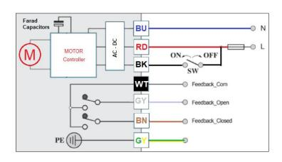
The actuator cable should come as a cut flying lead but may ship with our factory standard white PIN connector. Please remove and terminate as required. This fitting is purely for our test panels to enable quick testing of the product.
